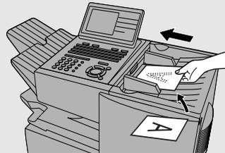
Note: When inserting a large number of pages in the feeder, slant the front end of the stack so that the bottom pages enter first.
