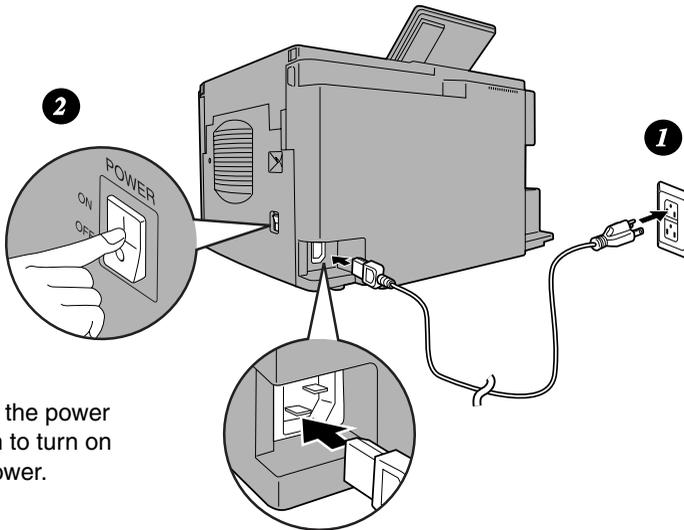
Press the power switch to turn on the power.
