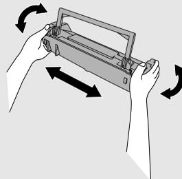
**7 Hold the toner cartridge by the handle and insert it into the print compartment.**
