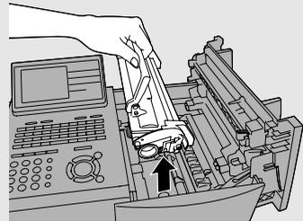
To make the cartridge more compact for disposal, press the buttons on the ends of the handle and fold the handle down.
