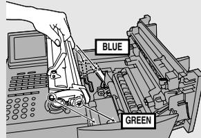
**7** If you have a paper cassette and the display still indicates that paper is jammed, pull out the cassette and remove the jammed paper.
