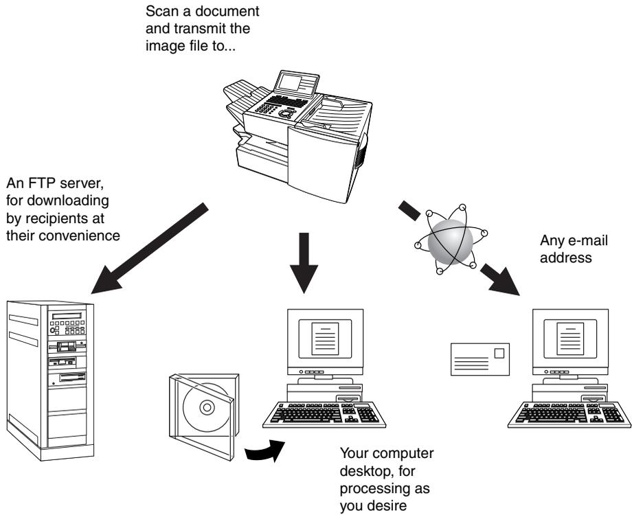
Scan destinations can be stored in Rapid Keys on the machine, for easy one-touch scanning and transmission.
