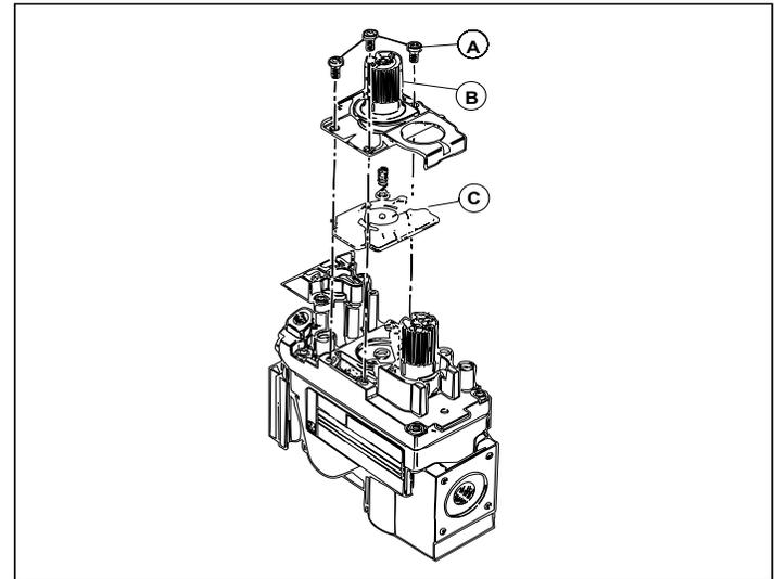
**Figure 6.6** Turn control knob to the OFF position, ensure that gas supply to the valve has been turned off. Using a Torx TH20, or slotted screwdriver, remove the three pressure regulator mounting screws (A), pressure regulator tower (B), and diaphragm (C).
