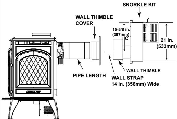
This is the only venting configuration that requires the use of the rear vent derating orifice that comes with the rear vent kit. **NOTE: A Snorkel Kit is required.**
