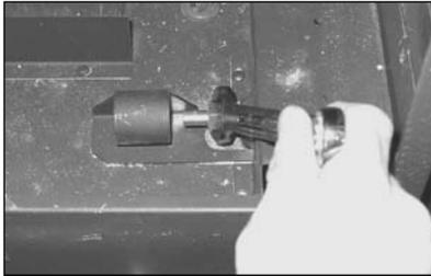
**Figure 6.5** Replace orifice with the proper size as indicated below for your gas type and venting. Re-install burner. Slide burner neck into shutter and over orifice. Re-install burner pan locators on left and right side of the burner. Secure with one screw to each side.
