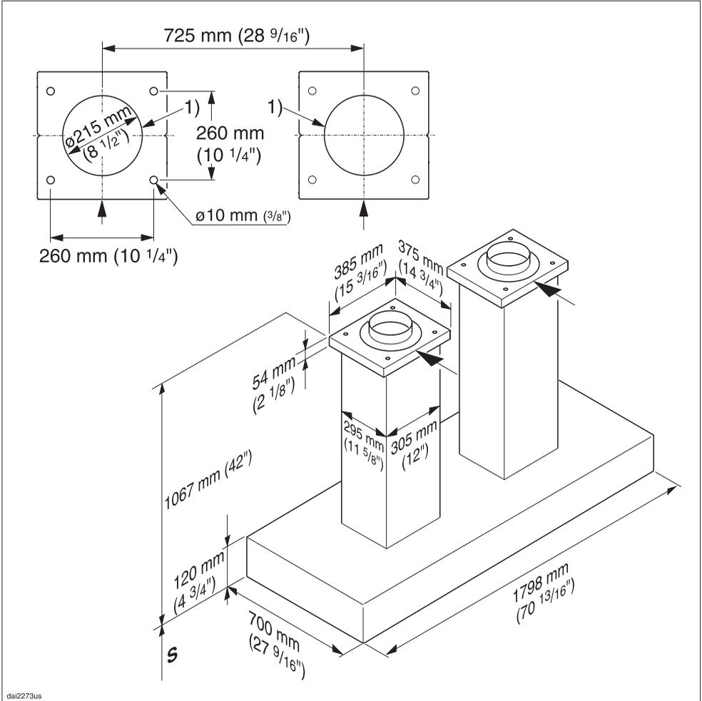
Exhaust connection 2 x 6" (2 x 150 mm) diameter
