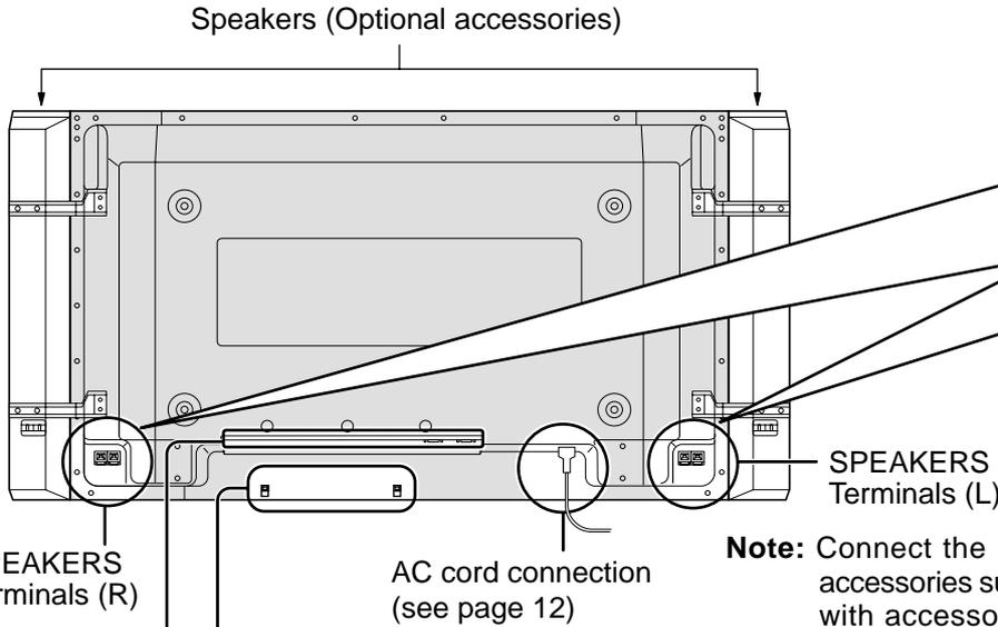
**Note:** Connect the power cord before combining with accessories such as the pedestal. When combining with accessories such as the pedestal, be very careful not to pinch the power cord.
