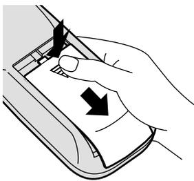
2. Install the batteries as shown in the battery compartment.
