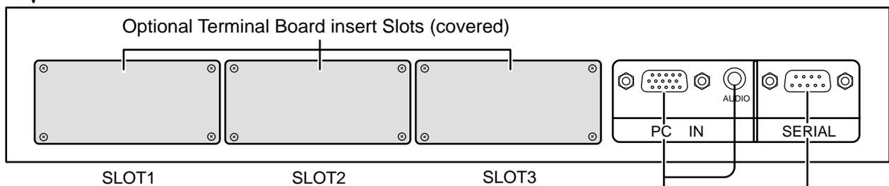
**Note:** Insert the optional terminal boards before combining the Plasma Display with the pedestal.
