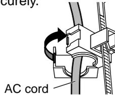
3. Slide up the clamber and fix the AC cord plug securely.
