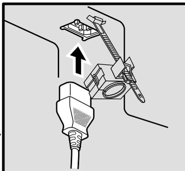
Fix the AC cord plug securely to the Plasma Display with the clammer. (see page 7)
