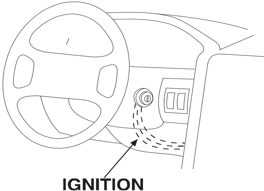
Once the lower dash panel has been removed, locate the ignition harness at the back of the key cylinder. This is usually a group of heavy gauge wires (approximate 14ga.).
