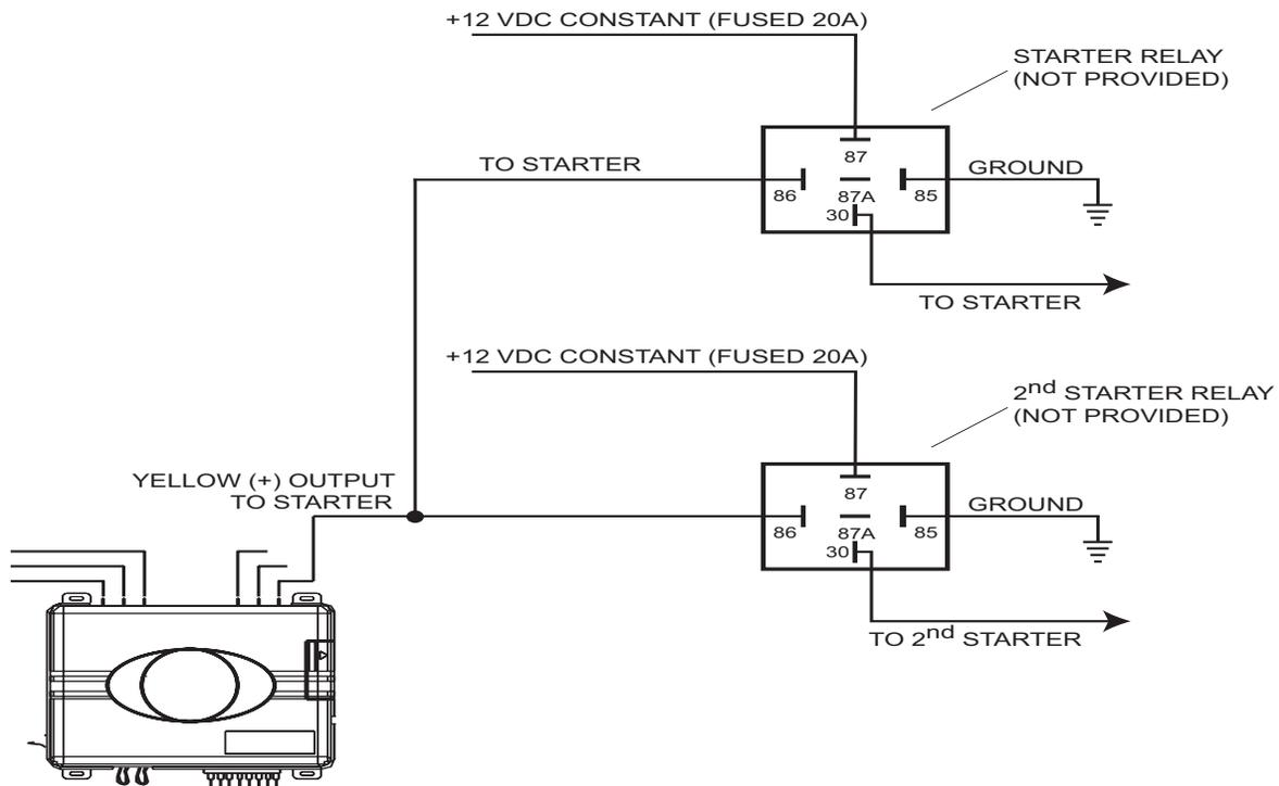
**note!** Always check the Web site information on your vehicle for warnings regarding the starter wire and check engine lights. Some vehicles will trip a check engine light if the starter wire is cut.
