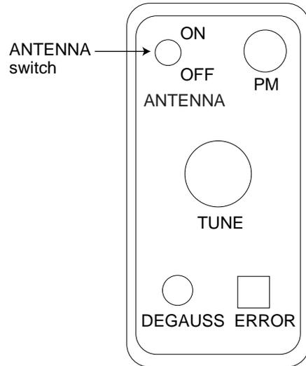
Figure 3-5 Antenna switch in tuning compartment
