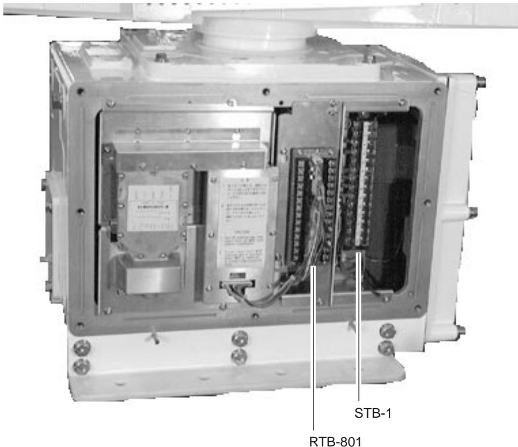
*Figure 2-10 Scanner unit, port side view*
