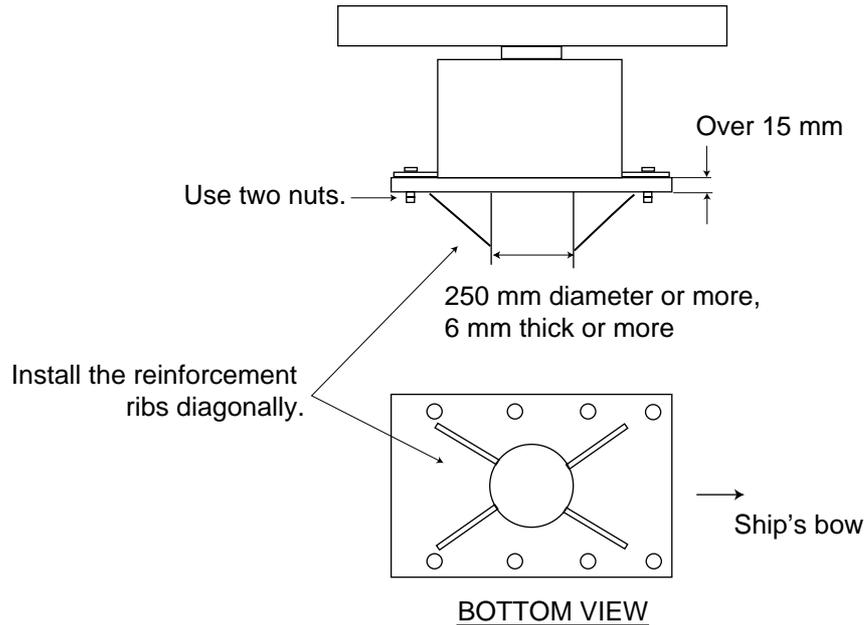
*Figure 1-5 Installation of reinforcement ribs*
