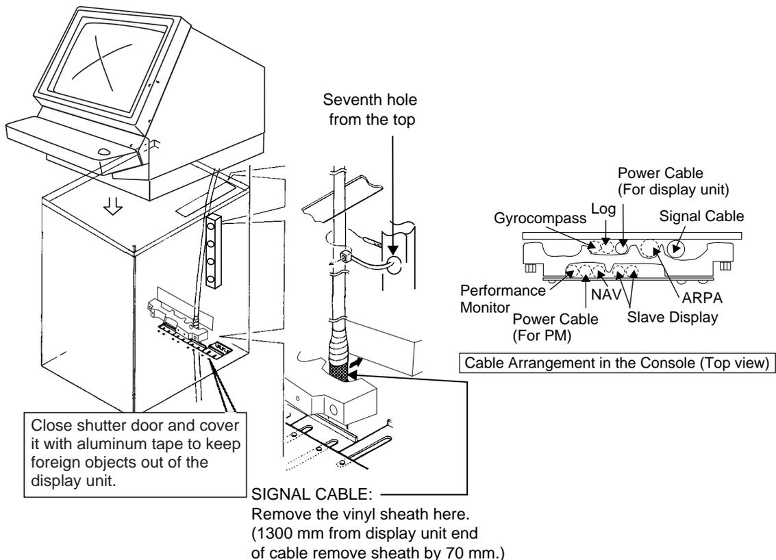
Figure 2-4 Clamp position at bottom of display unit
