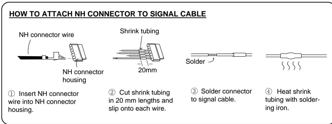
Figure 2-6 How to attach NH connector
