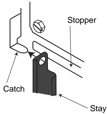
*Figure 1-10 Setting catch to hole in stay*
