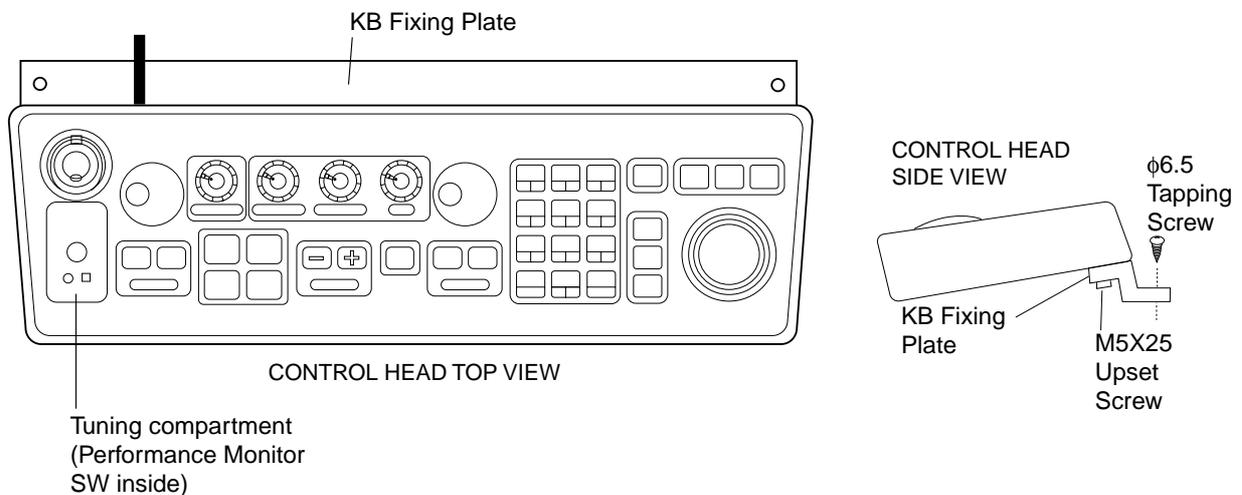
Figure 1-16 How to attach KB fixing plate
