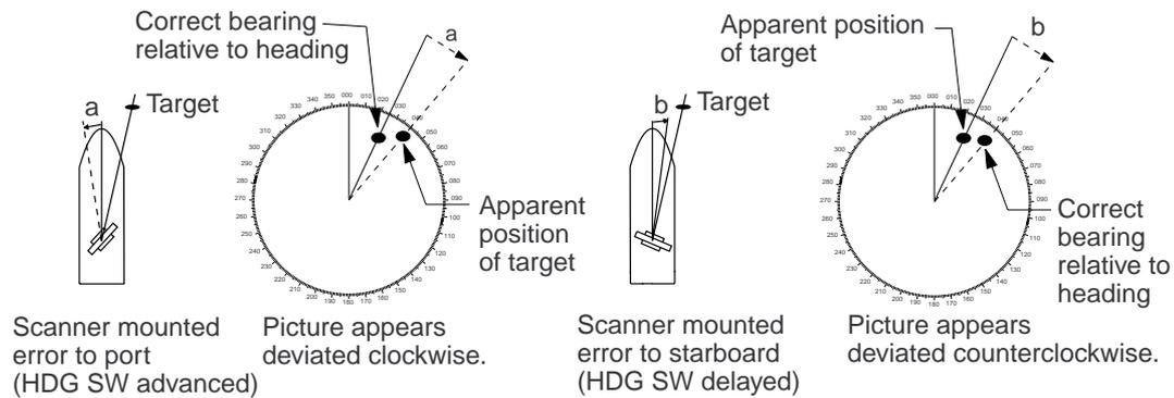
*Figure 3-2 Heading alignment*
