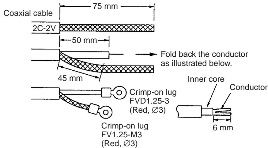
Figure 2-15 Fabrication of coaxial cable
