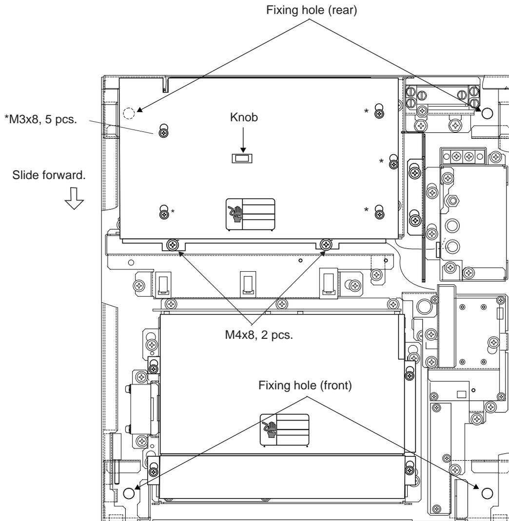
*Figure 1-12 How to remove the PTU cover*
