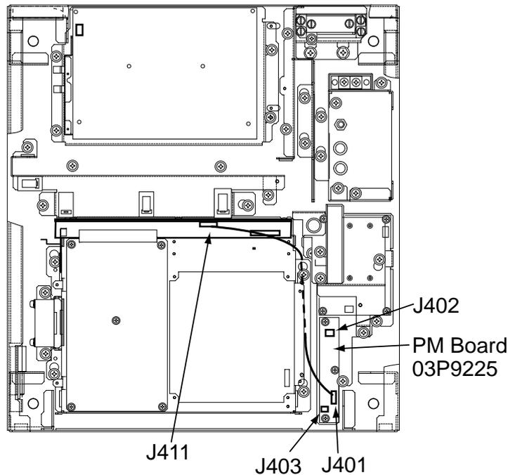
*Figure 4-15 Display unit, inside view*
