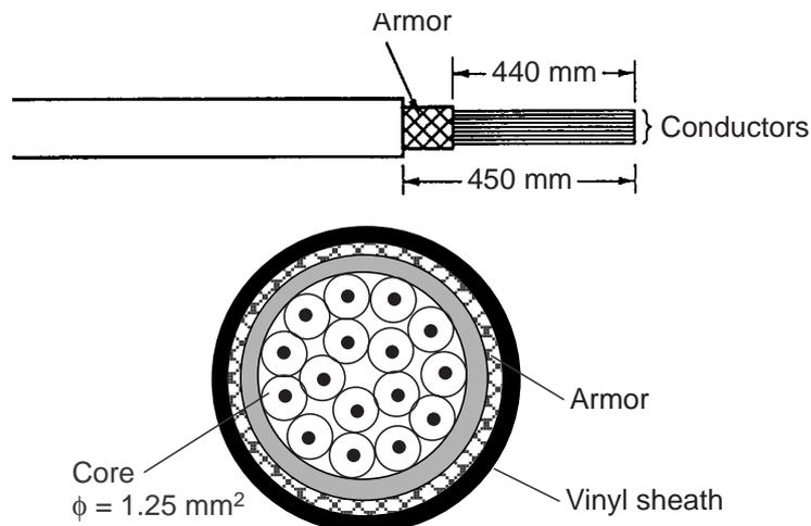
Figure 2-7 Fabrication of multicore cable 660V-MPYCY-12/250V-MPYCY-12
