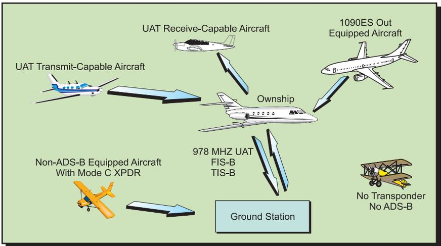
Figure 3-1 GDL 88 ADS-B In and Out
