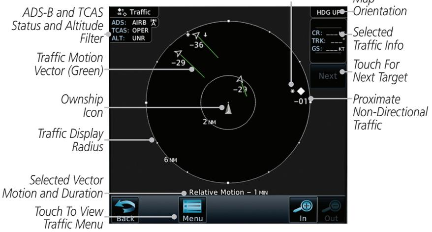
**Figure 4-2 AIRB Display with the GTN 7XX**
