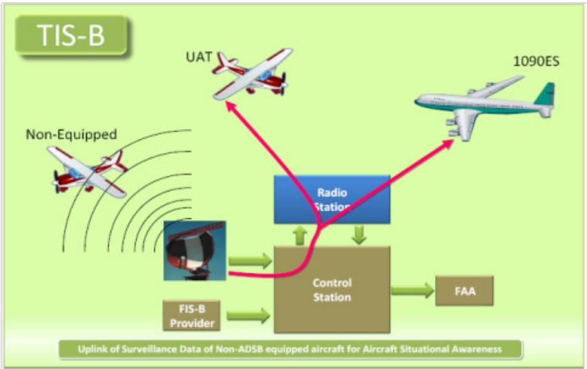
Figure 2-5 TIS-B Operation - FAA Illustration
