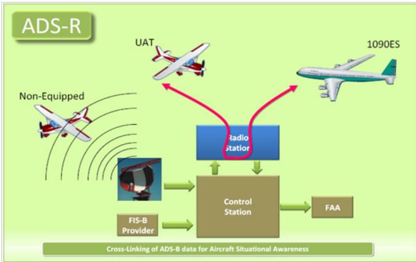
**Figure 2-4 ADS-R Operation - FAA Illustration**
