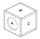
**Note:** All sealed box airspace should be filled to 50% loose poly-fil stuffing. Please allow two weeks of break-in time for the CompVR subwoofer to reach optimum bass performance.
