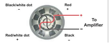
Series Wiring Dual 2  $\Omega$  = 4  $\Omega$  Load Dual 4  $\Omega$  = 8  $\Omega$  Load
