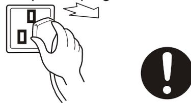
Do not damage the power cord, bend, extend, twist, bind or alter it by force. Do not press or nip it with weight. If the power cord or the power plug is bad, or the power plug becomes flexible, to avoid risk it is required to have it replaced by the technicians of our special shop or the after-sale service department. Keep the pin of the power plug clean, if the power plug is polluted with dust, please wipe with dry cloth carefully.
