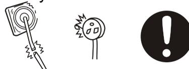
Do not put the machine at damp place like the bathroom. Never wash it with water. Not put wet laundries on the control panel.
