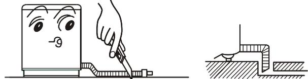
3. If the drain hose is too long , cut it at mid point. To make smooth drainage, cut the front end of the hose into slope.
