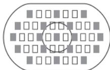
With the 39 AF points indicated by ■, high-precision, cross-type AF (both horizontal- and vertical-line sensitive) is possible during manual AF point selection. The cross-type sensors' vertical-line sensitivity is approx. two times higher than their horizontal-line sensitivity. The remaining six AF points will be horizontal-line sensitive.
