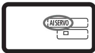
**This AF mode is for moving subjects when the focusing distance keeps changing. While you hold down the shutter button halfway, the subject will be focused continuously.**
