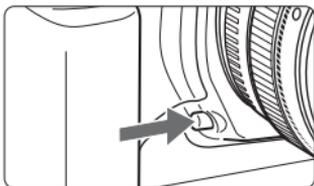
Press the depth-of-field preview button to stop down the lens to the current aperture setting. You can check the depth of field (range of acceptable focus) through the viewfinder.
