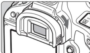
If you take a picture without looking at the viewfinder, light entering the eyepiece can throw off the exposure. To prevent this, slide the eyepiece shutter lever as shown by the arrow to shutter the eyepiece.
