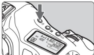
Press the <☀️> button to turn on (☀️6)/off the illumination of the top/rear LCD panel.
