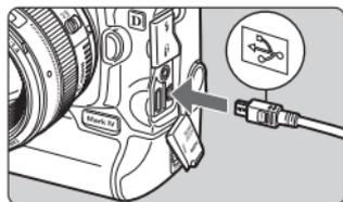
**3** Connecting the camera to a printer
