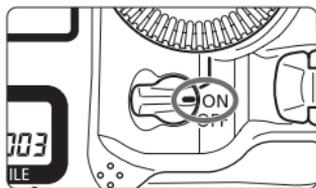
**5** Set the camera's power switch to <ON>.
