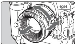
**While pressing the lens release button, turn the lens as shown by the arrow.**
