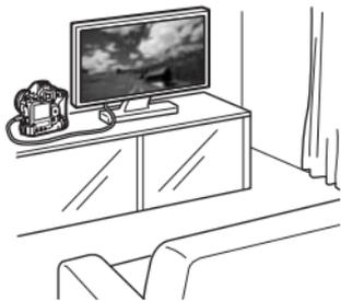
Use the provided stereo AV cable or HDMI Cable HTC-100 (sold separately) to connect the camera to a TV set. You can then playback the captured movies and photos on the TV.
