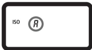
If the ISO speed is set to “A”, the actual ISO speed to be set will be displayed when you press the shutter button halfway. As indicated below, the ISO speed will be set automatically to suit the shooting mode.
