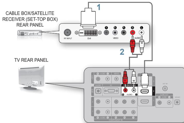
1. Connect an HDMI Cable (Not supplied) between the **HDMI IN 2** jack on the TV and the HDMI jack on the Cable Box/Satellite receiver (Set-Top Box).
