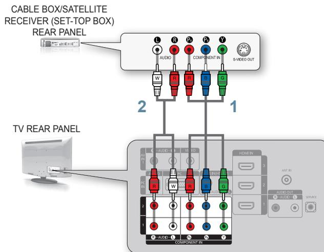
1. Connect a Component Cable (Not supplied) between the **COMPONENT IN (1 or 2) [Y, Pb, Pr]** jacks on the TV and the COMPONENT jacks on the Cable Box/Satellite receiver (Set-Top Box).
