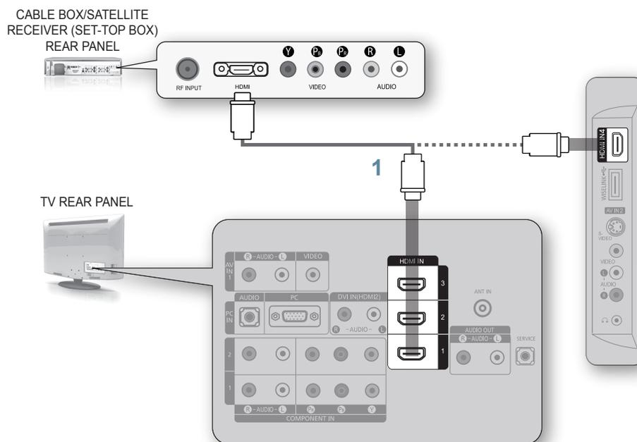
1. Connect an HDMI Cable (Not supplied) between the **HDMI IN (1, 2, 3 or 4)** jack on the TV and the HDMI jack on the Cable Box/Satellite receiver (Set-Top Box).
