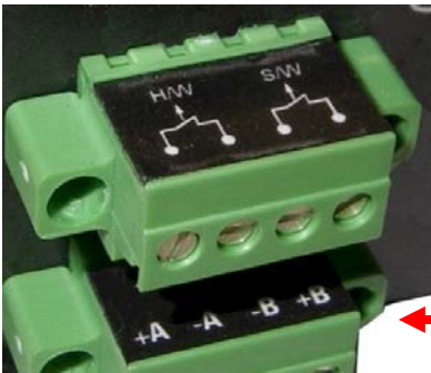
Figure C5.0: DC Dual-Source, wiring connections with Dual-Source option.
