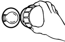
3. Turn bulb counterclockwise to remove from socket.
