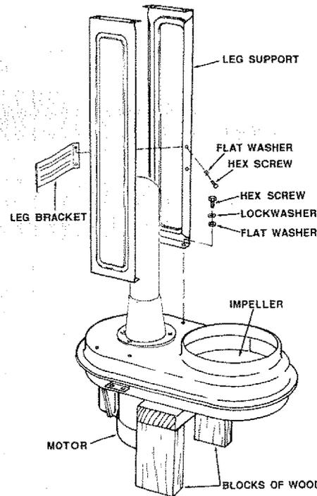
flange of *Leg Support* and attach to threaded hole of *Bracket*.
