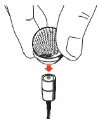
Please install the MZW 2 wind-shield, first. This wind-shield reduces the wind noise by a maximum of 20 dB.
