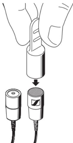
Please protect your MKE platinum-C by means of the makeup protection, if you attach your MKE platinum-C to your body and want to put on makeup. The makeup protection is easy to install: just slip it on the microphone (with or without slip-on cap). The makeup protection prevents makeup from penetrating into the gauze. Remove the makeup protection shortly before you enter the stage.
