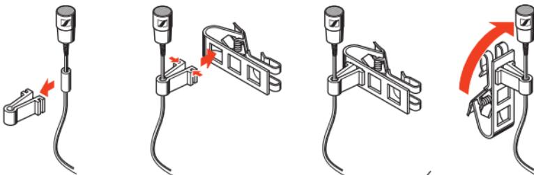
For thin clothes (e.g. silk), please use the outer hole where the clip's contact pressure is the highest.
