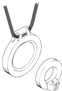
You may also use the ZH 102 pin to attach the microphone to articles of clothing made of fabric that will not be damaged by the pin. The pin attachment withstands high mechanical loads and is also a very convenient solution, if the articles of clothing do not have collars or edges to which the MZQ 02 clip can be attached.
