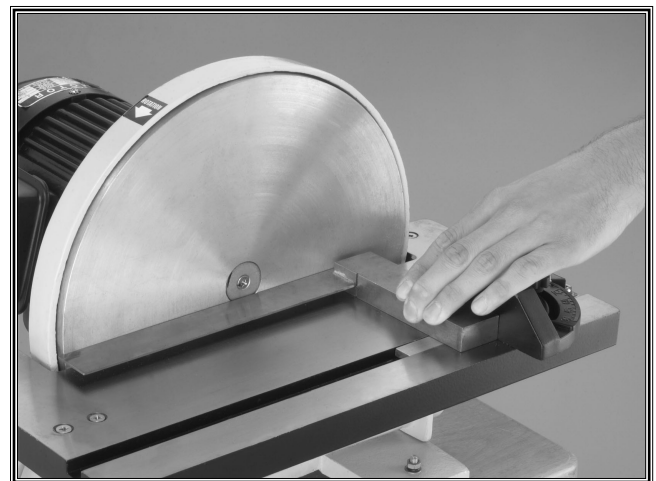
Figure 5. Checking table square.
