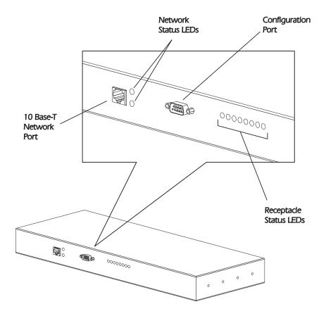
Figure 1: MasterSwitch Front Panel
