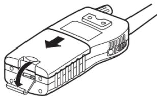
3. Insert 3 AA ALKALINE batteries according to the polarity symbols inside the battery compartment.
