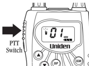
*Hold the radio with microphone approximately two inches in front of your mouth with the antenna at approximately 45° angle away from your head. Speak in a clear, normal conversational voice.*
