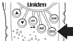
1. When **[SCAN]** SW is pressed during Group Scan Mode, **SCAN** icon will blink and Group Scan Scanning begins.
