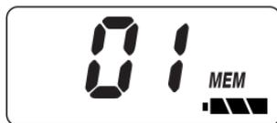
When the batteries in the unit are low, the unit will go into a Battery Low/Sleep Mode. The Scan Mode, Transmit, Transmit Call Tone Mode are disabled. Replace the batteries immediately to continue using the radio.
