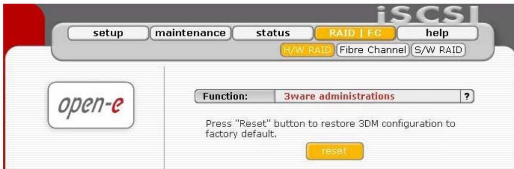
Please note that the RAID controller should be supported by the Open-E software. If a 3ware controller is installed you can click on RAID in the menu and the 3ware web base will start automatically.
