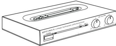
1. Fully extend the receiver's antenna.
