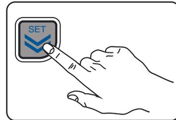
if a selection is not made after 15 seconds, the last value displayed will be confirmed automatically and the chamber temperature display is restored.
