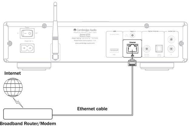
**Note:** Only connect the LAN port of the player to an Ethernet port that supports 10BASE-T or 100BASE-TX. Connecting to any other ports or jacks, such as a phone jack, can damage the unit
