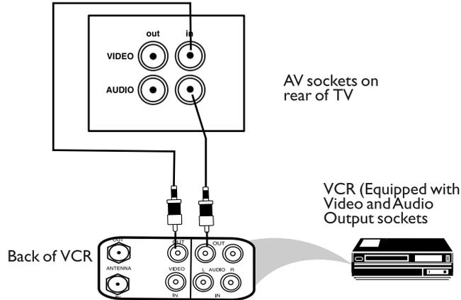
You can view the playback of VCR tapes (Video Disc players, camcorders, etc.) by using the AUDIO and VIDEO INPUT sockets on the rear of the TV.
