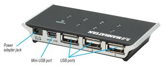
**NOTE:** The power consumption of each connected device is limited to 500 mA. If, after connecting the hub to the PCs, any of the ports fail to work normally, disconnect the device(s), as the failure may be due to excessive current. Reconnect the device(s) to allow the hub to recover and operate normally.
