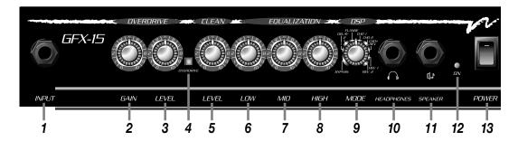
1: INPUT: Connect your guitar here by means of a shielded instrument cable.
