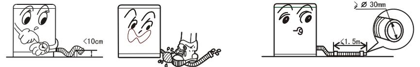
3. If the drain hose is too long, cut it at mid point. To make smooth drainage, cut the front end of the hose slantingly.
