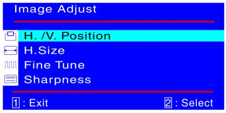
**Image Adjust :** To manually adjust the Horizontal /Vertical position ,H. Size, Fine Tune and Sharpness.
