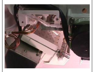
The ABS water plate sprays water up into the evaporator cells to form the square IM cube.
