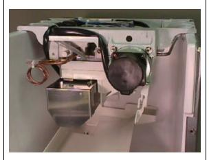
Unlike the initial harvest, the normal harvest is controlled by the thermistor. When the thermistor reaches 59°F, the control board deenergizes the hot gas valve and energizes the condenser fan motor. The actuator motor energizes to raise the plate. When the plate reaches the evaporator, the actuator toggle switch is moved back to the right. The board de-energizes the inlet water valve and the freeze cycle begins again. The average harvest cycle is about 3 minutes.
