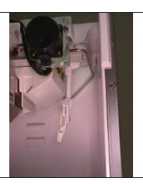
The IM51 uses a mechanical proximity switch bin control assembly located in the bin area.
