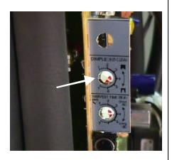
The board adjustments are made through variable resistors on the board. The cube control is marked VR5. This adjusts the thermistor switching temperature of - 9.4°F and the length of the freeze cycle. The dimple size in the cube also changes. Adjusting to a larger dimple will result in a shorter freeze cycle and a smaller cube. A smaller dimple setting will result in a longer cycle and a larger cube. The factory setting is 5.
