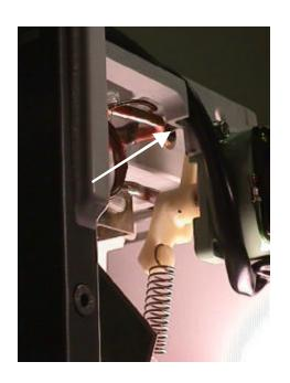
The front cam arm has a switch lever that operates the actuator toggle switch located above the pan assembly.
