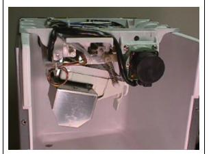
The moveable water pan assembly includes the water plate, reservoir pan, and pump motor assembly.
