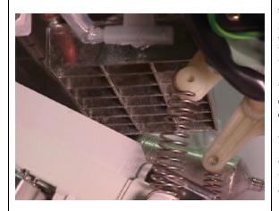
A thermistor temperature of  $-9.4^{\circ}F$  signals the control board to begin harvest and energize the hot gas valve and actuator motor circuit. The actuator motor now turns counter clock wise to lower the water pan. The switch lever moves the actuator toggle switch to the left. This sets the actuator motor circuit to raise the water plate at the end of harvest. The board energizes the inlet water valve.
