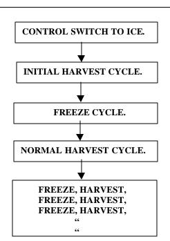
Now, lets take a look at the basic IM sequence of operation. When the control switch is placed in ICE, the unit starts in the Initial Harvest cycle.
