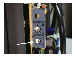
The defrost control VR2 will adjust the time period between ice-drop and actuator motor restart during harvest. The factory setting is 4. This setting represents approximately 40 seconds. VR2 would be adjusted longer if the unit is operating in a cooler ambient temperature.
