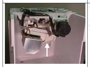
Switching the actuator toggle switch to the left position also reverses the actuator motor. The motor now turns clock wise to raise the water plate upward.
