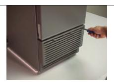
The louver covers the compressor compartment. Remove the louver screws and lift the louver forward to access the condenser coil fan assembly and compressor.
