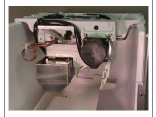
When the plate reaches the evaporator, the cam arm switch lever moves the actuator toggle switch to the right position. This stops the actuator motor and sets up the circuit to lower the plate in the next harvest cycle. It also energizes the pump motor and the board de-energizes the inlet water valve. The Freeze Cycle now begins.
