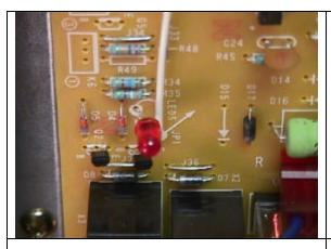
A red Service Indicator LED is also included on the control board. This LED will either light continually or flash to indicate a service fault. A fault diagnosis chart in the service manual will help the technician determine the actual problem.
