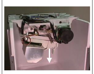
The actuator motor turns counter clock wise to rotate the cam arms and lower the water pan away from the evaporator. When the water plate is completely down the switch lever moves the actuator toggle switch to the left. The board energizes the inlet water valve and condenser fan motor and de-energizes the hot gas valve.
