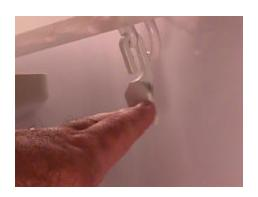
When ice fills the bin and pushes the control arm over, the activator magnet moves to the switch and closes the contacts.
