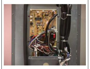
A solid state board controls the IM operation. Several adjustments are included on the board. These adjustments are factory set for proper operation.
