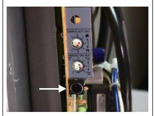
The control board includes a pushbutton reset. Pressing this button will initiate a harvest cycle anytime the control switch is in ICE position.
