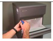
Access to the evaporator compartment is gained by removing the front and top covers.
