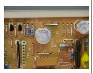
The maximum freeze timer is VR3. This timer will automatically switch the unit to the harvest cycle if the freeze cycle last longer than the setting time. The factory setting is 45 minutes.
