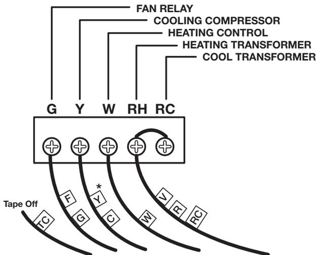
\* If both Y and C wire are present, tape off "C" wire.
