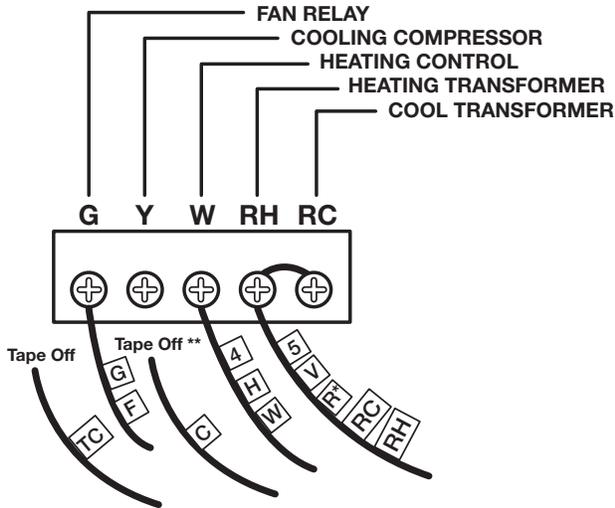
\* If replacing a Honeywell TM-11, tape off wire "R"; connect wire "B" to terminal "RH."
