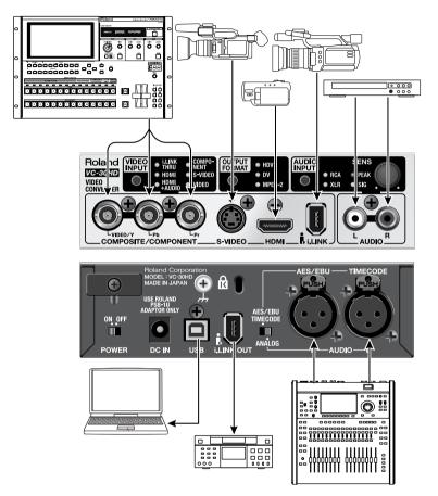
This unit is equipped with balanced XLR type jacks. Wiring diagrams for these jacks are shown below. Make connections after first checking the wiring diagrams of other equipment you intend to connect.
