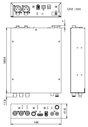
\* When using the holes in the side panel to secure the unit in place, use screws measuring 3 mm in diameter and whose length is no more than 8 mm from the surface of the side panel.
