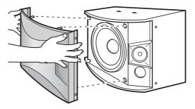
To reattach, do these steps in reverse order. The 4 pegs inside the grille should be set in the corresponding holes on the speaker.
