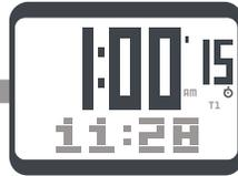
After 1 hour, the resolution switches to 1 second for up to 100 hours
