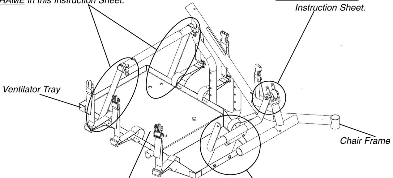
*C. Refer to INSTALLING THE VENTILATOR TRAY ONTO THE CHAIR FRAME in this Instruction Sheet.*
