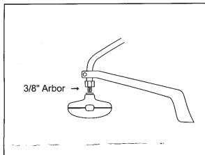
After removing original head (unscrew counterclockwise), replace with No-Brainer™ quick load head. Ready to use.
