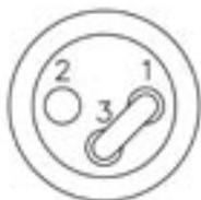
On the XLR connector pin 1 is ground, pin two is positive input and pin 3 is inverted (negative) input. Pin numbers are marked on the XLR. If you re-install the jumper incorrectly or leave it lying about, the amplifier will not work properly, and you will be able to tell.
