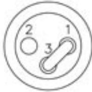
On the rear panel you will find both RCA and XLR type input connections for single-ended or balanced inputs. If you use the RCA input, be certain that the XLR connector has a gold shorting plug between pins 1 and 3, which connects the “minus” input to ground, otherwise the amplifier will not operate properly. If you lose this shorting plug, just contact the factory – we give them away all the time.
