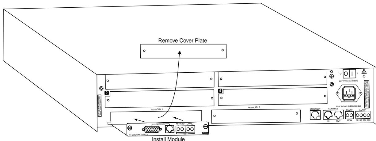
Figure 1. Installing the T1 Network Interface Module
