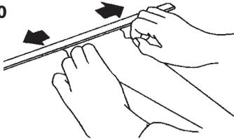
2. Remove the saturated grease filter.
