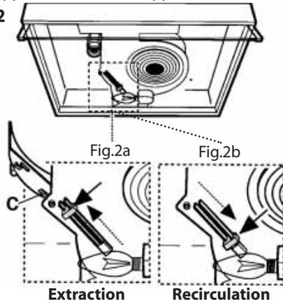
**NOTE: The hood is more efficient in the exhaust mode, therefore this position should be selected during the warmer months of the year when no heating is being used. When the room is being heated, if the recirculation position is selected heat will not be wasted.**
