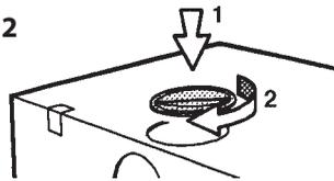
Place the new carbon filter, ensuring that it is aligned. To lock the filter turn in the direction of the arrow (Fig.13)
