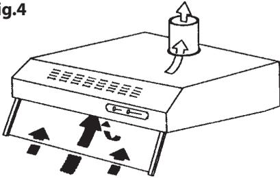
If the exhaust air is being drawn upwards, a pipe with a diameter of 100mm is necessary and the blanking plate must be fitted in the rear outlet. To check that the hood is set up for extraction, open the grille panel and make sure that the conversion lever on the unit is in the exhausting position.
