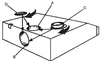
This method is recommended if at all possible. Fumes and grease laden air are drawn into the underside of the hood and expelled out.
