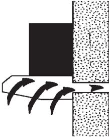
If the air is to be drawn off to the rear, a pipe with a diameter of 100mm is necessary and the blanking plate should be fitted in the top outlet.
