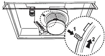
The Hood must not be connected to ducting when in the recirculating mode. Regular replacement of the charcoal filter will ensure optimum performance from the hood when recirculating.
