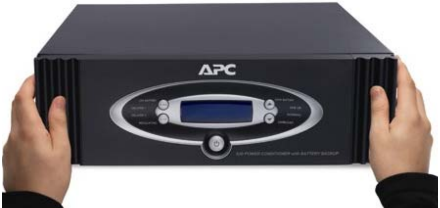
Figure 4. Front Bezel Removal
