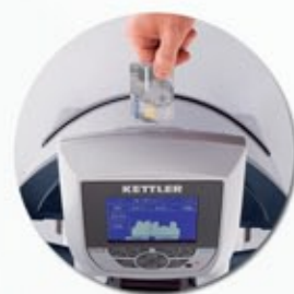
Training computer with chip-card reader for storing user-specific data.
