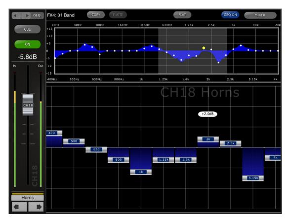
The current channel's Name, Color, Fader, Level Meters, [ON] and [CUE] buttons are shown in the left column. At the bottom-left, there are "previous" and "next" arrow buttons for navigating to different channels. Pressing these buttons will only access other channels that have GEQs assigned to them.
