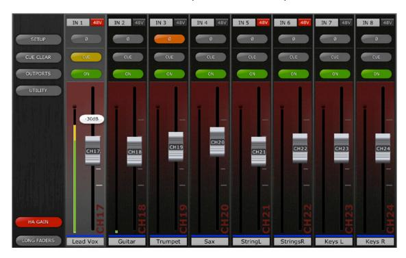
Faders can be moved to change the HA Gain for each channel. The gain value of each head amp will be displayed above the fader while any fader cap is being touched. Up to 8 faders can be adjusted simultaneously.
