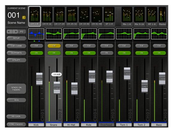
Across the top of the screen, level meters and faders are displayed in blocks of channels for mono Input Channels 1-48, Stereo Input Channels 1-4, Mix and Matrix busses, and the Master Stereo and Mono busses. This is the "Navigation/Meter Bridge".
