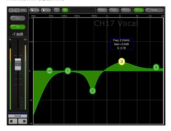
The current channel's Name, Color, Fader, Level Meters, [ON] and [CUE] buttons are shown in the left column. At the bottom-left, there are "previous" and "next" arrow buttons for navigating to different channels.
