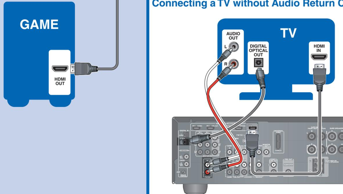
When there is no OPTICAL output in the TV, connect the analog output. The function of HDMI THRU, Power Control and TV Control can be used by turning on HDMI Control (RIHD) from the setup menu.
