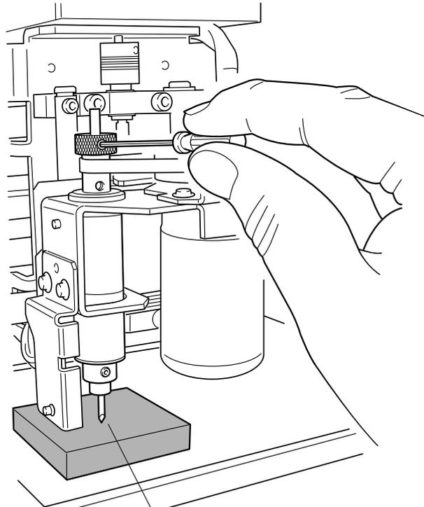
Loosen the retaining screw for the cutter holder and move the cutter until it touches the material.
