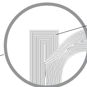
The spacing of these lines is the pitch.
