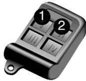
Pressing Buttons I and II at the same time will begin the remote start sequence. The parking lights will flash to confirm that the motor is going to start. It is important to release the transmitter buttons as soon as
