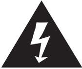
The lightning flash with arrowhead symbol, within an equilateral triangle, is intended to alert user to the presence of uninsulated "dangerous voltage" within the product's enclosure that may be of sufficient magnitude to constitute risk of electric shock to persons.
