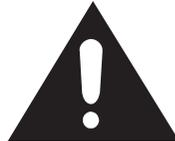
The exclamation point within an equilateral triangle is intended to alert user to the presence of important operating and maintenance (servicing) instruction in the literature accompanying the appliance.
