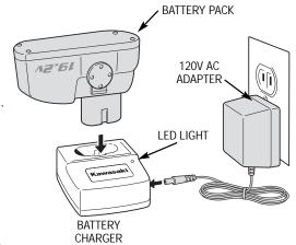
3. When fully charged, reattach battery pack onto Cordless Tool, making certain latches fasten securely. Cordless Tool will not operate properly if the battery pack is not seated properly.
