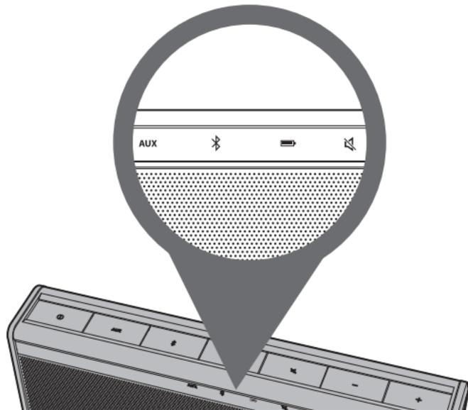
**AUX** The speaker is playing the source connected to the AUX (⊕) input.
