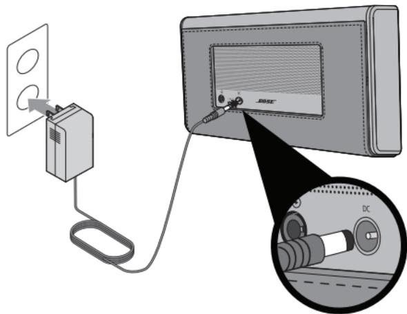
3. Plug the power supply into a live AC (mains) outlet.
