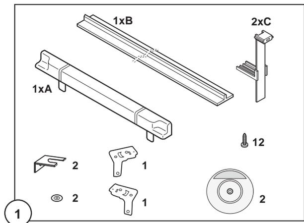
3. Two cabinet securing brackets are supplied with the installation pack. They need to be assembled onto the cabinet prior to cabinet being pushed into the Kitchen aperture.
