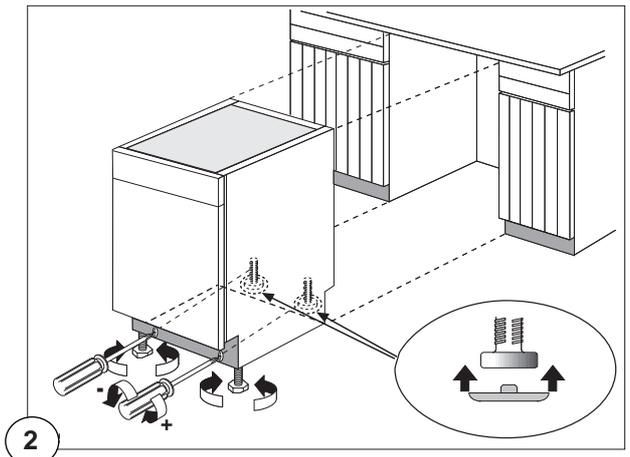
6. If necessary, pads are supplied for the rear feet to make sliding the appliance in and out of the recess easier. To fit the pads, press them onto the rear feet.
