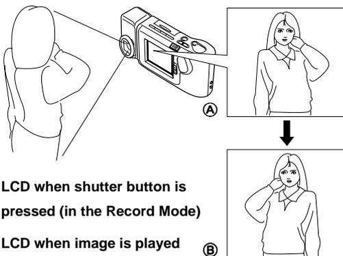
**A** ..... LCD when shutter button is pressed (in the Record Mode)
