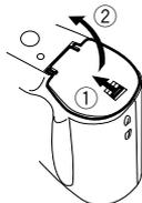
2. Insert four batteries and close the battery compartment cover.
