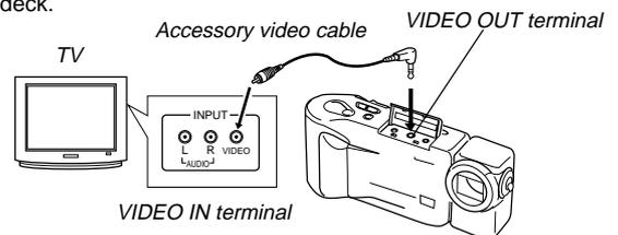
After connecting the camera and TV, set the channel of the TV to the channel used for video input.
