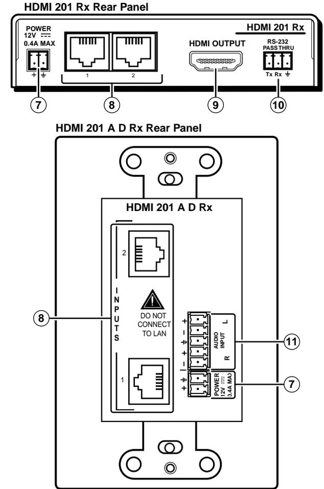
**Figure 2-16 — HDMI 201 Rx rear panel connectors**
