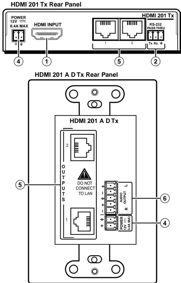
**Figure 2-13 — HDMI 201 Tx rear panel connectors**
