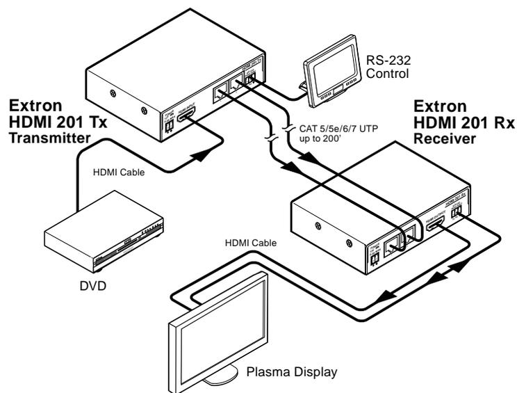
**Figure 1-1 — Typical transmitter and receiver application**
