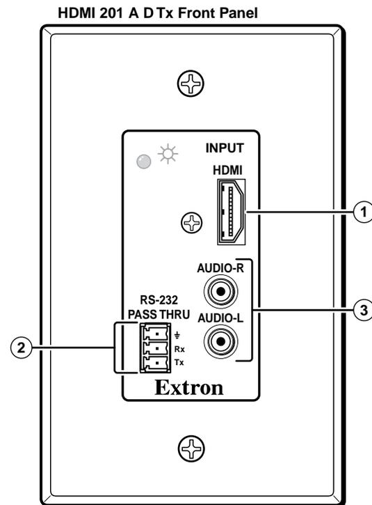
**Figure 2-12 — HDMI 201 Tx front panel connectors**
