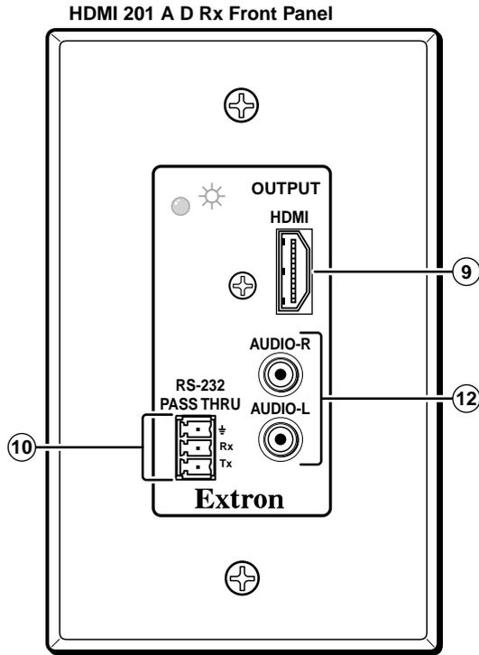
**Figure 2-17 — HDMI 201 A D Rx front panel connectors**
