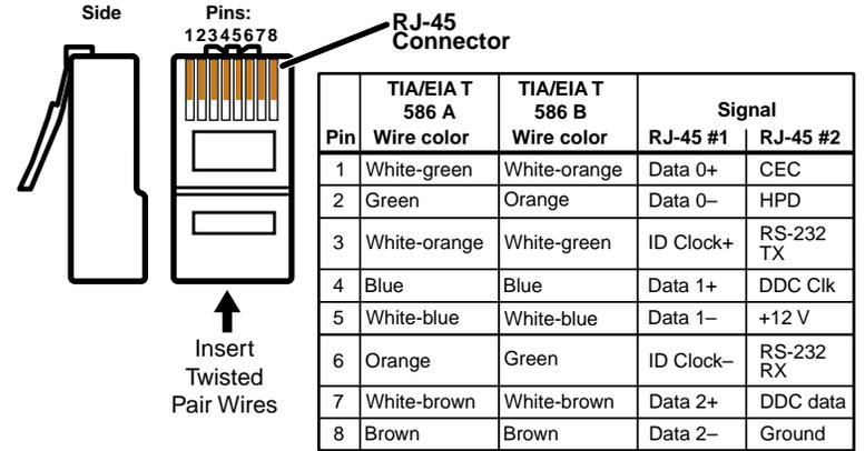
**NOTE** Terminate both ends of both cables identically, in accordance with either the TIA/EIA T 568A or the TIA/EIA T 568B wiring standard.
