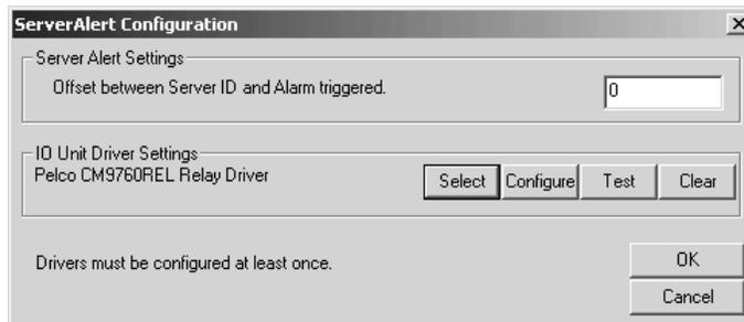
**Figure 100.** Relay Unit Driver Settings Dialog Box
