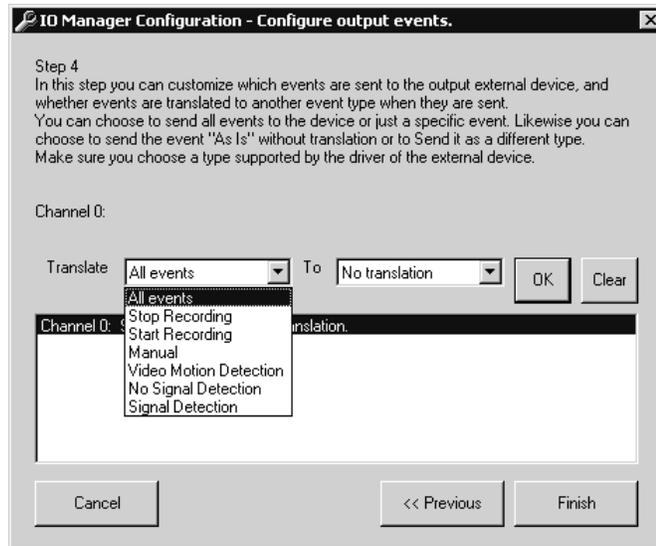
**Figure 83.** Dialog Box to Configure Relay Event Type
