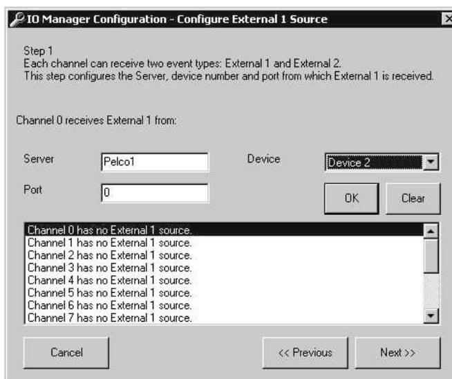
**Figure 74.** Dialog Box to Configure External 1 Source
