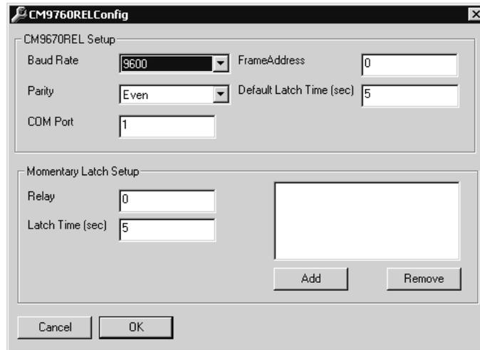
**Figure 81.** CM9760 Relay Configuration Dialog Box
