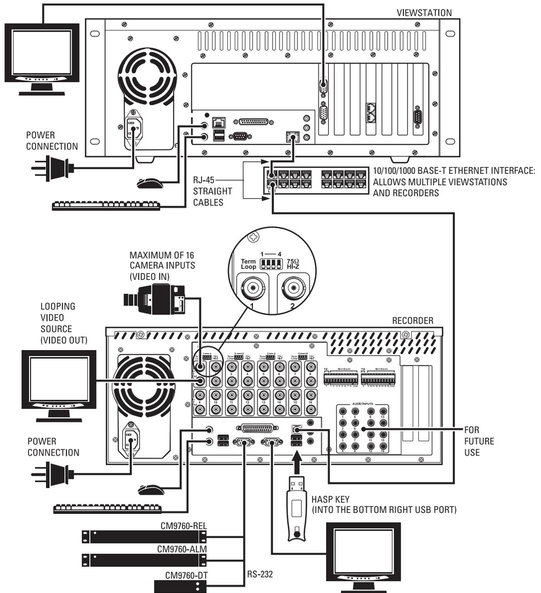
**Figure 8. System Connections**
