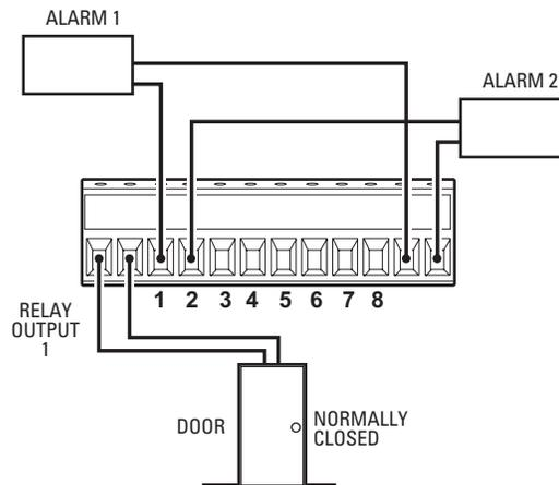
**Figure 9.** Alarm and Relay Wiring
